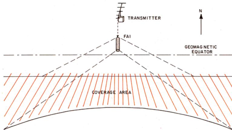
**Fig. 4** When a station north of the equator is transmitting in a southerly direction, the southern coverage area will be similar to that shown in this drawing, shown as if looking down from a great height. Size of this area is dependent upon the length and horizontal extent of the scattering medium, and its position relative to the transmitter and receiver. The coverage pattern for a southern station beaming north would be a mirror image of that shown here.
