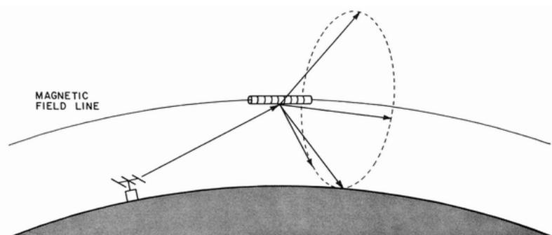
**Fig. 3 - This diagram gives an example of ray scattering. Irregularities aligned with Earth's magnetic field are illuminated by a radio wave. Energy is scattered back to Earth in a cone-shaped pattern. Stations within the area intersected by the cone can receive the signal.**
