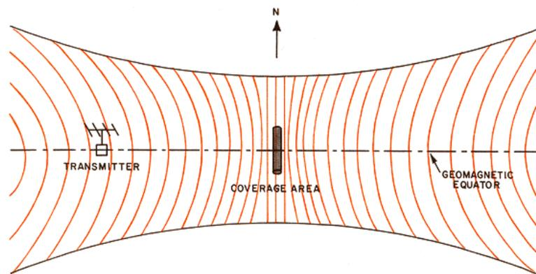
**Fig. 5** Scatter-mode coverage in an east-west direction along the magnetic equator. As in the case shown in Fig. 4, coverage area is dependent upon the horizontal extent of the scattering medium. A relatively wide coverage area may be possible if north-south alignment of the irregularities is not an important aspect of the phenomenon.
