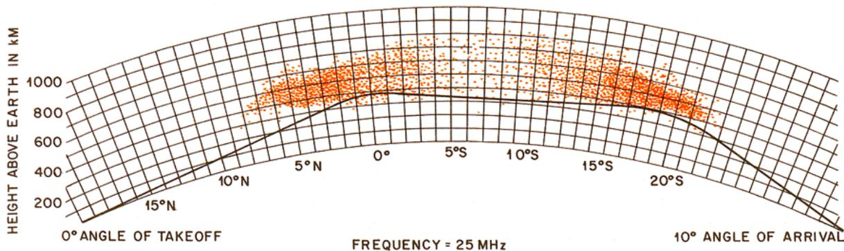
**Fig. 2 - Cross section of a transequatorial ray path, showing the effect of ionospheric tilt on a 25 MHz signal. This drawing shows a typical example of TE propagation. (From Davies, "Ionospheric Radio Propagation," U.S. Government Printing Office, Washington, DC 1965.).**
