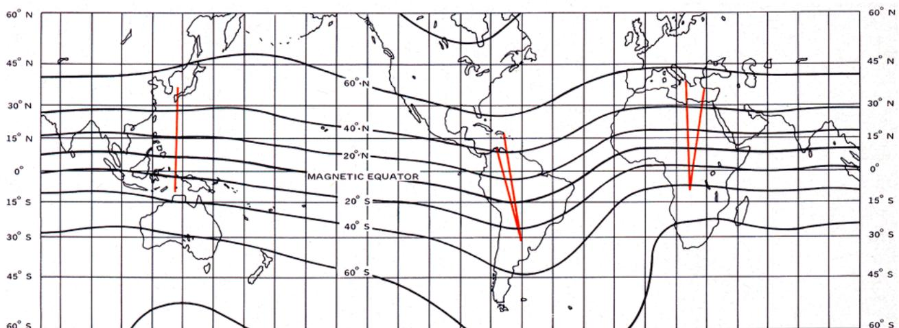
Fig. 1 - Approximate location of stations which successfully made use of FAI can be seen on this map. The contour lines indicate geomagnetic latitudes.
