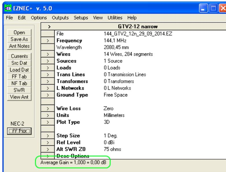
If the bent DE's tubes are tapered using a stretch of 10 mm in diameter in the middle and fitting 8 mm tubes into it to the sides, NEC will not handle the tapered sections correctly.
