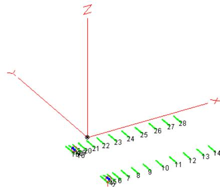
**Step 4:** Last we copy the 2 Yagis using 'Offset copy Z by' 3,558 mm.
