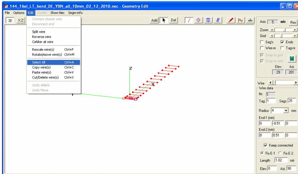
Use *menu => Edit => 'Select All'*. Move and copy Yagi(s) using window *'Rotate and Move'* above *'Select All'*. *'Move'* is self explaining whereas *'Create n new structs'* is what is called *'Copy Wires'* in EZNEC. Fill in '1' for a single copy and a number for displacing distance on the right axis. Before next *'Move'* command make sure to have selected all new and old wires you want to move. Repeat *'Select All'* or mark by hand using *'ctrl'* and mouse clicks.
