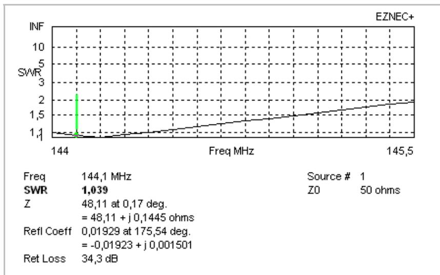
However, VE7BQH uses just the real part, the resistance R picked from complex impedance  $\underline{Z}$  for the G/T table. It will not make a significant difference what figure to use as long as the Yagi is not far from the wanted impedance. Since small angles  $\varphi$  provide very small changes only. => Consequently we note 48.1 Ohm as our Z for the G/T table.
