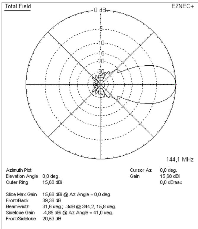
Azimuth Plot of a GTV 2-12n
