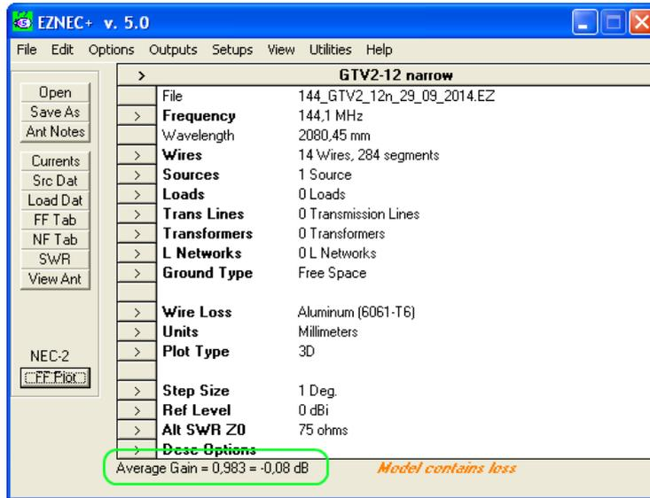
It must be mentioned that since the basis for setting up the G/T table is the NEC2 Kernel as used in EZNEC or standard 4nec2 installations, it is of no help if a model with too high AG computes correctly in any other advanced antenna design program. It may prove the model to be fine in general but does not help in putting up a table on an equal base since the NEC2 based EZNEC would still deliver overoptimistic results in relation to the other Yagis enclosed in the G/T table.
