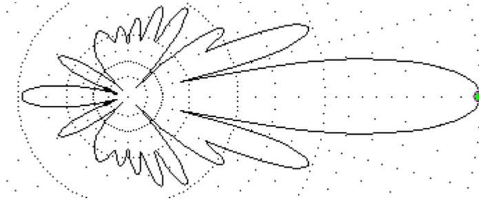
Pic.: Elevation Plot - 16 elem. GTV 2-16 (DG7YBN) bay over stacked by 0.4 m
