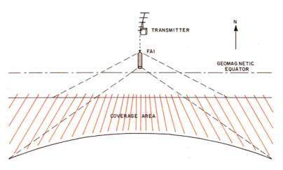
Fig. 4 When a station north of the equator is transmitting in a southerly direction, the southern coverage area will be similar to that shown in this drawing, shown as if looking down from a great height. Size of this area is dependent upon the length and horizontal extent of the scattering medium, and its position relative to the transmitter and receiver. The coverage pattern for a southern station beaming north would be a mirror image of that shown here.
