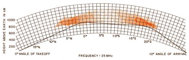
Fig. 2 - Cross section of a transequatorial ray path, showing the effect of ionospheric tilt on a 25 MHz signal. This drawing shows a typical example of TE propagation. (From Davies, "Ionospheric Radio Propagation," U.S. Government Printing Office, Washington, DC 1965.).
