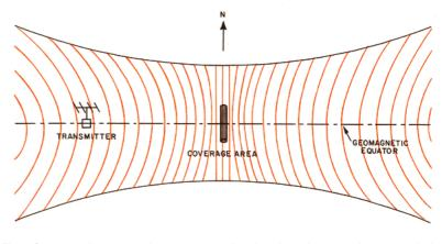
Fig. 5 Scatter-mode coverage in an east-west direction along the magnetic equator. As in the case shown in Fig. 4, coverage area is dependent upon the horizontal extent of the scattering medium. A relatively wide coverage area may be possible if north-south alignment of the irregularities is not an important aspect of the phenomenon.
