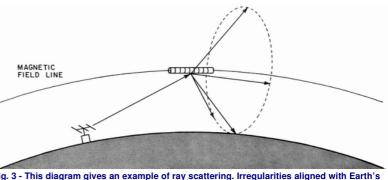
Fig. 3 - This diagram gives an example of ray scattering. Irregularities aligned with Earth's magnetic field are illuminated by a radio wave. Energy is scattered back to Earth in a cone-shaped pattern. Stations within the area intersected by the cone can receive the signal.
