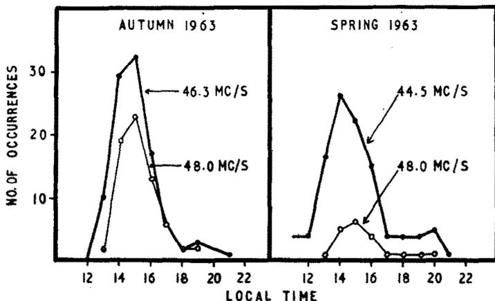
Fig. 3. Comparison of actual number of occurrences of LRTE during (a) Autumn 1963 and (b) Spring 1963 at the frequencies indicated.
