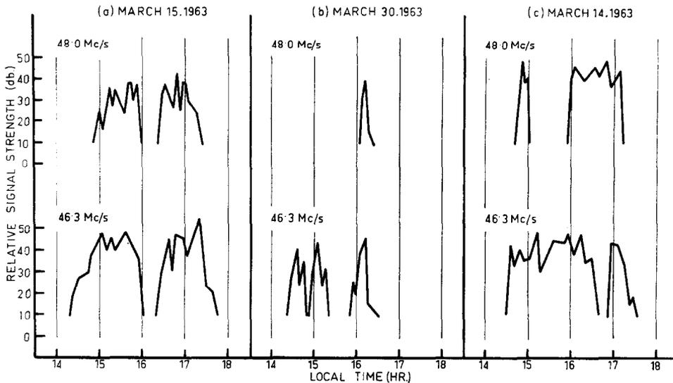
Fig. 5. Strength of Korean LRTE signals received at two frequencies at Townsville during Autumn 1963.
