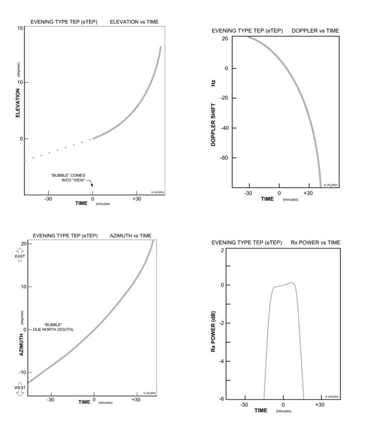
*Figure 3* diagrams re-traced. Note: these show 'ideal', smoothed, characteristics calculated from the numerical model, which are applicable to a frequency of 100 MHz.
