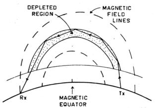
Figure 2. The wave-guide structure of the field-aligned interhemispheric equatorial plasma bubbles.
